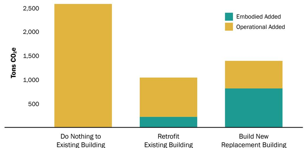
**FIGURE 12** This example of a summary chart from the 2Build or not 2Build Carbon Calculator illustrate that in the near term when carbon reductions are critical, reusing and upgrading an existing building can reduce total carbon emissions compared to new construction through avoided embodied emissions and reduced operational emissions.
