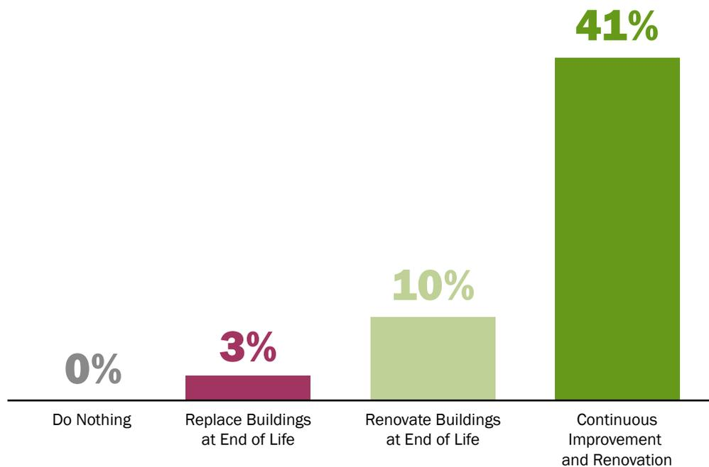
**FIGURE 19** This chart looks at the information from Figure 18 a different way. Each bar here shows the total percentage reduction in carbon emissions of each portfolio scenario compared to the baseline case in which no buildings are upgraded or replaced. While each of these scenarios could lead to carbon neutrality by the year 2037, this chart shows that how net zero is achieved has a substantial impact on the environment.
