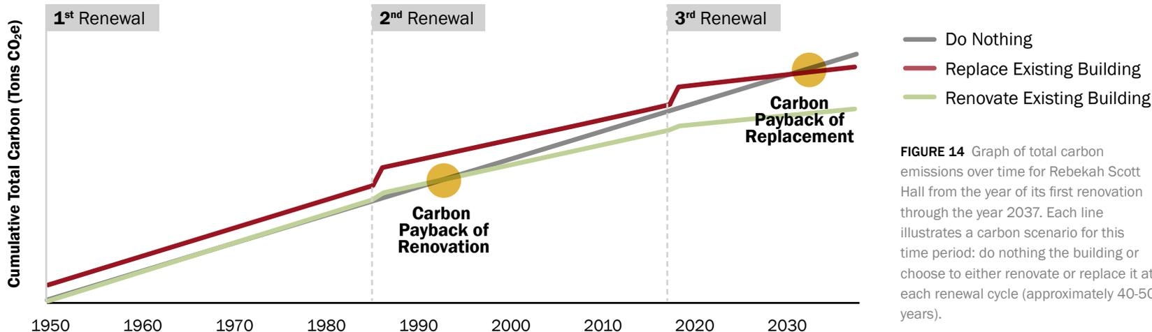
**FIGURE 14** Graph of total carbon emissions over time for Rebekah Scott Hall from the year of its first renovation through the year 2037. Each line illustrates a carbon scenario for this time period: do nothing the building or choose to either renovate or replace it at each renewal cycle (approximately 40-50 years).
