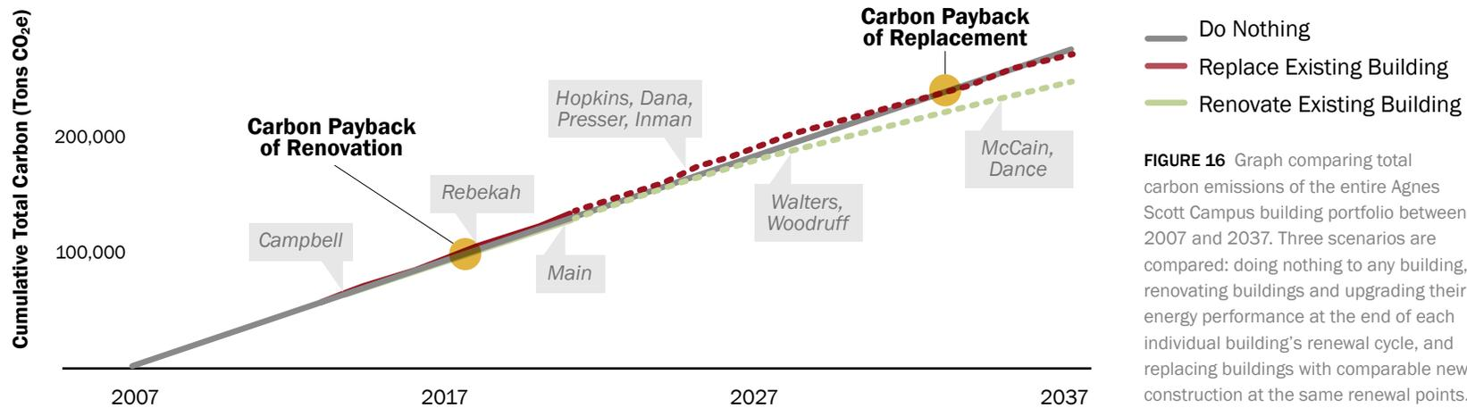
**FIGURE 16** Graph comparing total carbon emissions of the entire Agnes Scott Campus building portfolio between 2007 and 2037. Three scenarios are compared: doing nothing to any building, renovating buildings and upgrading their energy performance at the end of each individual building’s renewal cycle, and replacing buildings with comparable new construction at the same renewal points.
