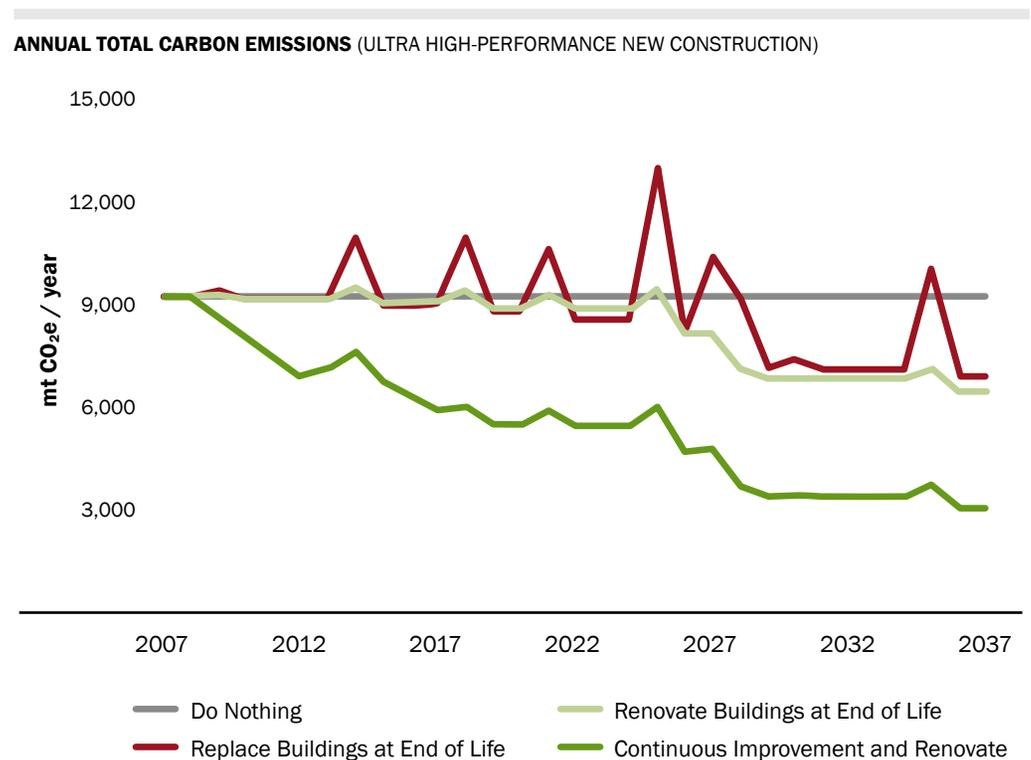
**FIGURE 18** This graph illustrates the trajectory of annual total carbon (embodied + operational) for four scenarios. The upward spikes indicate the one-time embodied carbon debt associated with new construction or renovation, while the decreasing slope represents reduced operational emissions over time. The area under each of these curves represents the cumulative tonnes of carbon emitted between 2007 and 2037 for each of these scenarios.
